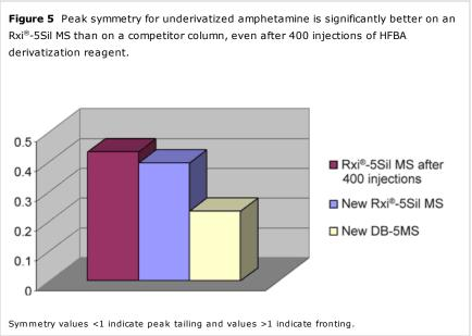
The rugged arylene phase of the Rxi®-5Sil MS column results in highly stable performance, even under the most demanding of analytical conditions, and its exceptional inertness ensures good peak shape for reproducible quantitation. The stability of the Rxi®-5Sil MS column results in longer column lifetimes, reducing both downtime and replacement costs.
