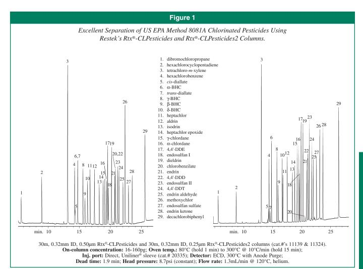
flow into the two columns with a glass 'Y' Press-Tight® connector, these chromatograms were acquired simultaneously.
