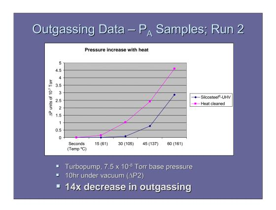
At hour 10 of pumpdown on a turbopump system, the Silcosteel-UHV coating still shows a significant improvement over a Heat Cleaned part. Base pressure is now in to the 10<sup>-8</sup> Torr range.
