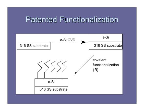
The basic Siltek process is sketched out here. An additional bonding to the surface (covalently) can further deactivate the surface. The beauty of this process, however, is that the "R" group can be a wide variety of molecules, thereby allowing tailorability of the surface to a customer's needs. For example, a fluorinated hydrocarbon can be bonded to increase hydrophobicity.
