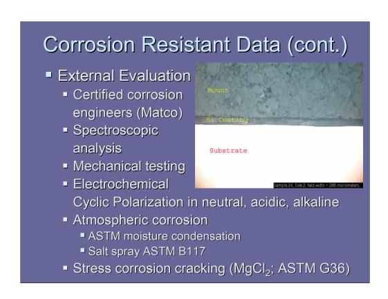
We use external experts for most of our data generation. For corrosion, several standardized tests were performed by Matco corporation.
