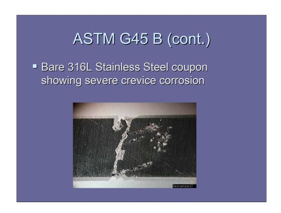
The location of the tight gasket is obvious in this photo of the uncoated coupon. Severe pitting corrosion is also present.
