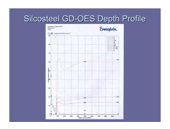
Using Glow Discharge Optical Emission Spectroscopy, a depth profile with real-time atomic percentage during the sputter shows atomic mixing of iron and silicon. This intimate mixing explains the absence of delamination with the silicon coatings. This is unlike polymeric coatings and provides a significant advantage over them.
