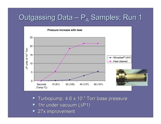
The treated parts were tested for outgassing rates after 1hr and 10hrs of pumpdown. This figure illustrates a significant decrease of outgassing rate when comparing the heat cleaned part to Silcosteel-UHV. Note the operating base pressure of  $4.6 \times 10^{-7}$  Torr.
