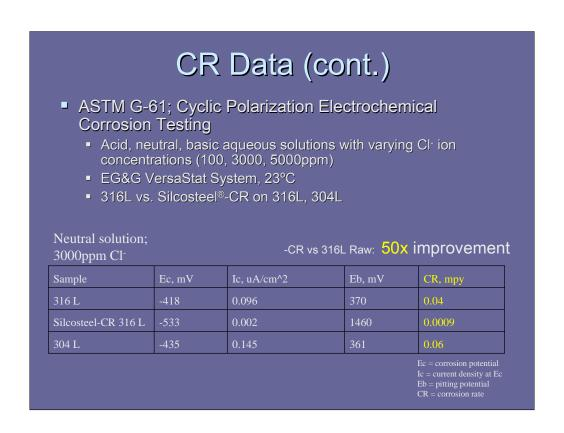
CP testing in neutral solution with 3000ppm Cl- gave a 50-fold improvement over an uncoated coupon.
