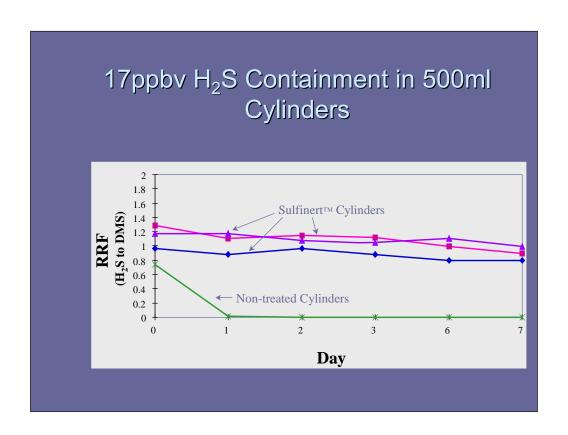
The following slides show data which highlight the inertness of the Siltek/Sulfinert surface. H2S is one of the most difficult sulfur gases for low-level transfer and containment, as it is highly adsorptive and reactive with a stainless steel surface. Here we show zero-to-negligible loss of 11ppbv H2S in a static storage cylinder over seven days.
