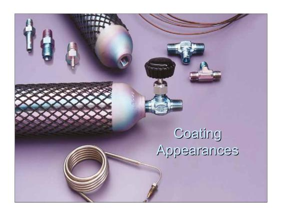
"Rainbow" coatings are approximately 1200A. Blue coatings range from 300-400A. Matte silver coatings are 1-10um. Tubing is generally coated only on the inside, whereas 3-dimensional parts are coated throughout all exposed surfaces, inside, outside, through pores and on fine structure.
