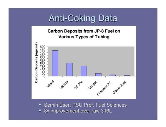
Comparisons of different surfaces shows a significant advantage of a coated substrate over other options.
