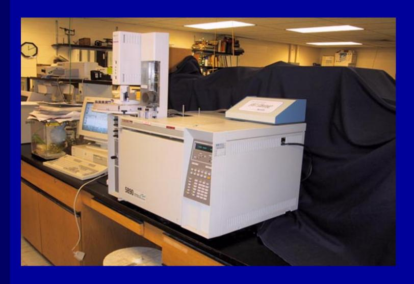
Restek Www.restekcorp.com GC Racer Installed on an Agilent 5890
