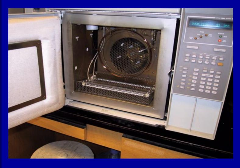
GC Racer Heater Installed in an Agilent 5890
