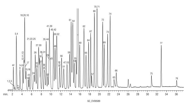
Experimental Fluorinated Polymer "Tail" 60m, 0.53mm, 3.00µm
