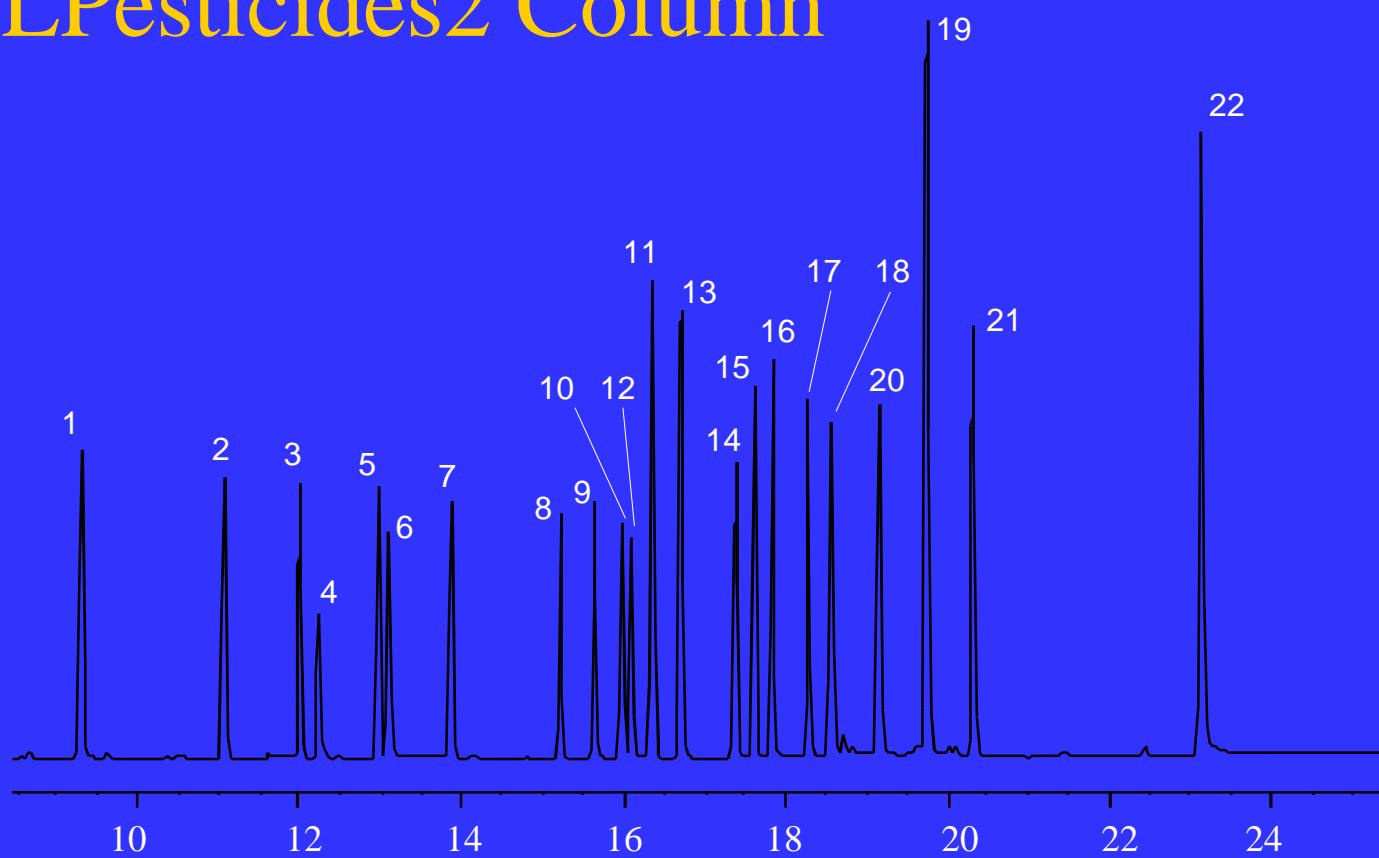
30m, 0.32mm ID, 0.25 $\mu$ m Rtx<sup>®</sup>-CLPesticides2; EPA 8081 list, direct Uniliner<sup>®</sup> sleeve (cat. #20335). Oven temp.: 120°C (hold 1 min.) to 300°C @ 9°C/min. (hold 10 min.); Inj. temp.: 200°C; Dead time: 1.797; Head pressure: 5.0psi (constant); Flow rate: 2.1mL/min. @ 120°C.
