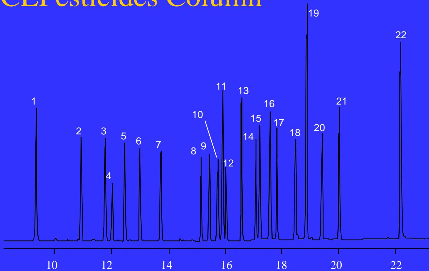
30m, 0.32mm ID, 0.5 $\mu$ m, Rtx<sup>®</sup>-CLPesticides; EPA 8081 list, direct injection, Uniliner<sup>®</sup> liner (cat. #20335). Oven temp.: 120°C (hold 1 min.) to 300°C @ 9°C/min. (hold 10 min.); Inj. temp.: 200°C; Dead time: 1.797; Head pressure: 5.0psi (constant); Flow rate: 2.1mL/min. at 120°C.
