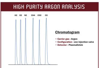
The combination of the PlasmaDetek and the high performance diaphragm valve bring outstanding measurement performance. A longer useful time and better performance on common GC techniques are achieved. They also allow new methods that are not possible with other commercial detectors and valves.
