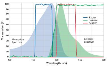
Typical measured CFP-3035D Filter Set for Green Fluorescent Protein. Hard-coating technology combined with single-substrate filter construction results in the highest transmission and steepest edges available.
