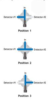
Characteristics of Manual Sample Injection Valves
