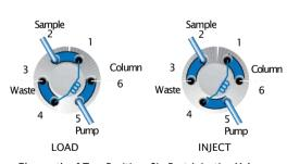
Flow path of Two-Position, Six-Port Injection Valve
