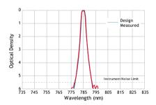
These graphs demonstrate the outstanding performance of the 785 rm MaxLine laser-line filter, which has transmission guaranteed to exceed 90% at the laser line and 0D > 5 blocking less than 1% away from the laser line. Note the excellent agreement with the design curves.
