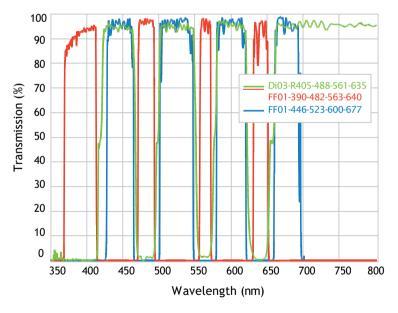
BrightLine multi-band 1/2 flatness super-resolution laser filter set, optimized for 405, 488, 561, and 635 nm laser sources.
