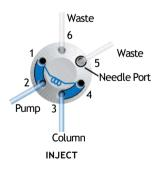
Flow path for the typical dual mode injector
