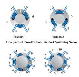
Flow path of Two-Position, Ten-Port Switching Valve
