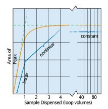
Figure 2 Sample mass (observed peak area) vs. volume of sample dispensed from the syringe, in units of loop volumes, injected onto the column from our dual mode injector such as model 7725
