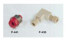
Thread PEEK Bulkhead Unions directly through your equipment housing to connect internal tubing to the outside. Each union has unique 3/8-24 external threads and comes complete with a stainless steel nut and lock washer to hold it in place. Requires a 3/8" hole to mount. The recommended torque limit for these unions is 15 in.- lbs (1.7 N·m).
