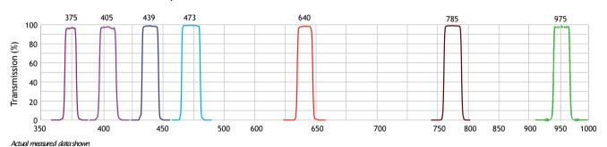
MaxDiode Filter Blocking Performance (470 nm filter shown)
