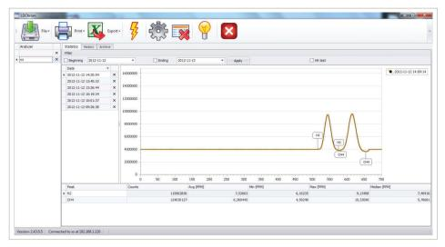
With the LDchrom data storage software, the chromatograms can be store at the user's convenience. It can generate reports, trend the detector signals and oven temperatures. All data can be saved and export to Excel. Offering its multiple modes, LDchrom can acquire data from multiple Multidetek configurations.
