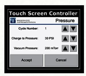
An on-board touch screen embedded controller makes the system operation as easy as pressing start. The controller allows the user to save up to ten different methods. The user can define each method including: Number of Cycles, Pressure, and Soak times. Once the method has been defined, it is saved and is accessible for later use.
