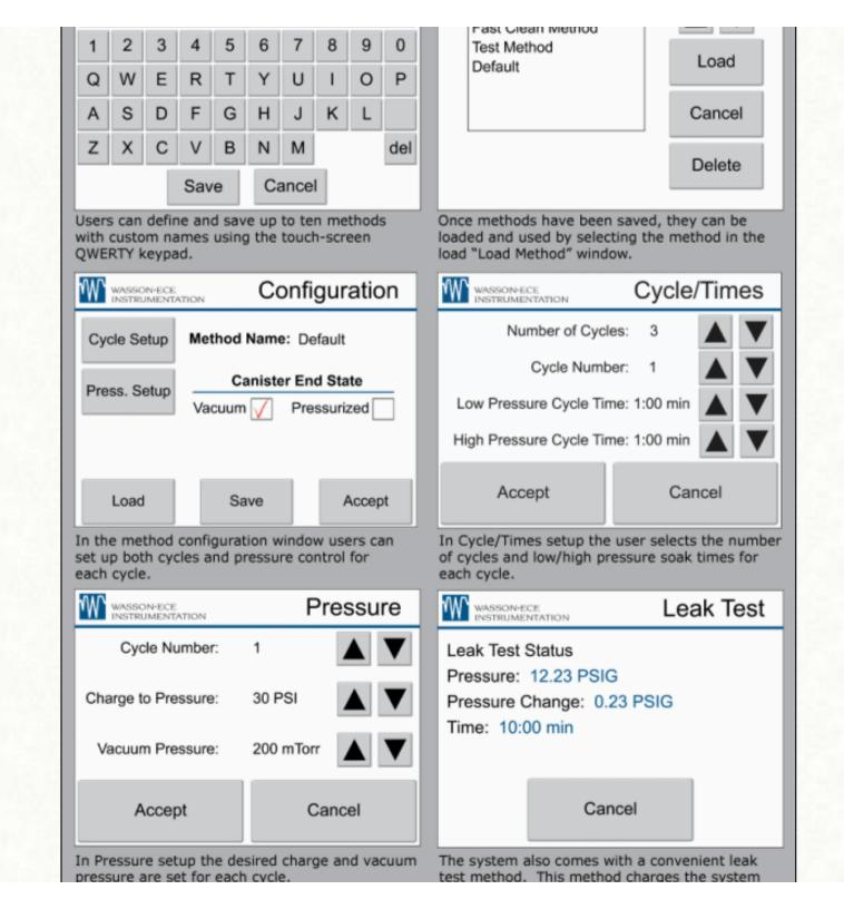
and looks for a pressure change over time indicating the system has a leak.
