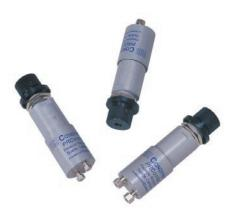
The VICI combo regulator is a combination regulator and shut-off valve. The pressure is set using the screwdriver adjustment in the center of the on/off knob. Turning the knob counterclockwise provides positive shutoff, while clockwise rotation restores gas pressure to within 0.05 psi of the setpoint.
