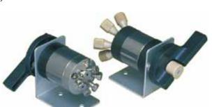
Direct syringe loading with a C1 injector allows a choice between the partial-filling method, in which the injection volume is determined by a syringe, and full-loop injection, in which the volume is determined by the size of the loop. A sample loop is supplied with the injector.
