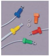
The basic component of the Cheminert system is the polypropylene nut, retained on PTFE or FEP tubing by a flange formed with a Cheminert flanging tool (page 70). This is an excellent method for connecting fluorocarbon tubing, as there is no reduction of the inside diameter and no binding or twisting of the tubing when the fitting is tightened. A mating of the parts is achieved with zero dead volume, making this an ideal fitting for biological systems.
