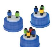
The VICI cap is the most economical way to helium sparge and deliver HPLC mobile phases. The insert is manufactured from PTFE, with a polypropylene screw cap and an EPDM\* O-ring which is resistant to commonly used HPLC solvents.
