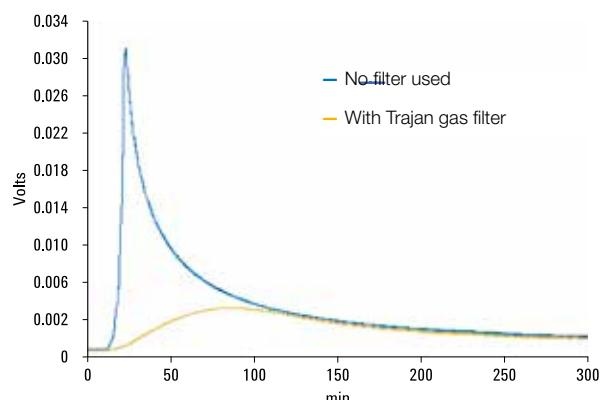
Figure 2 shows the difference in bleed levels of two GC columns due to moisture exposure with and without a filter when running a temperature program ( $50^\circ\text{C}$  to  $350^\circ\text{C}$ ,  $20^\circ\text{C}/\text{min}$ ). When no filter is used, an extreme rise in the bleed profile is clearly visible due to moisture in the carrier gas. By using gas filters, a normal bleed profile is achieved with the removal of all moisture in the carrier gas.
