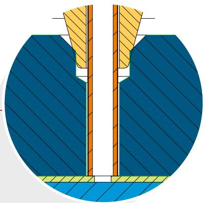
Fused silica to SilFlow connection system using SilTite FingerTite metal ferrule
