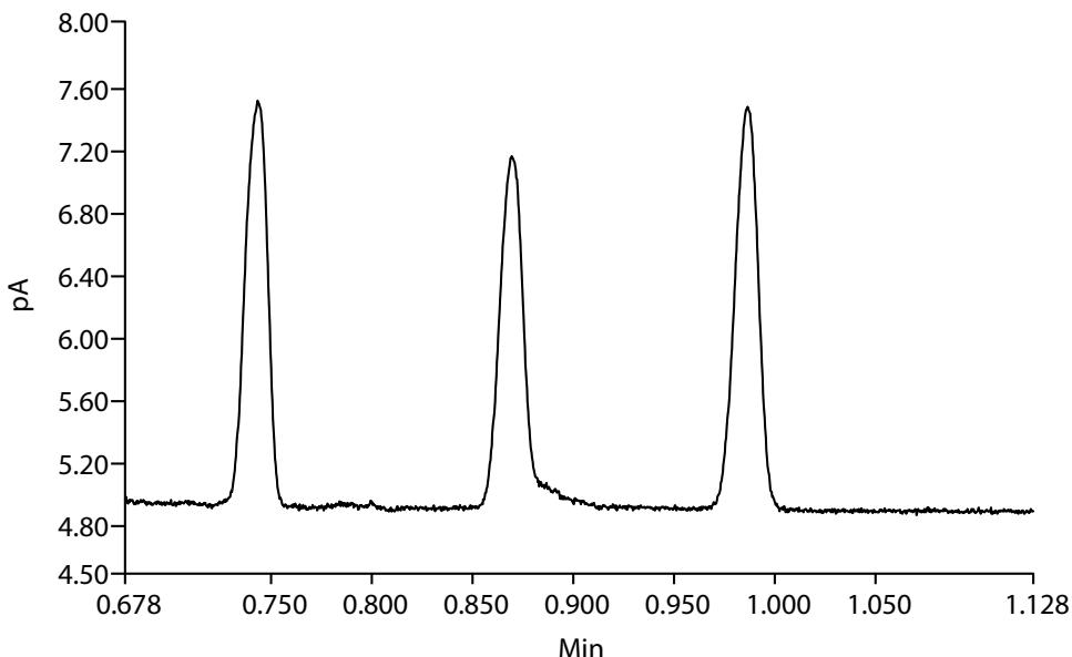
1  $\mu\text{L}$  expands to 432  $\mu\text{L}$ : Good peak shape, but approaching limits of half total liner volume.
