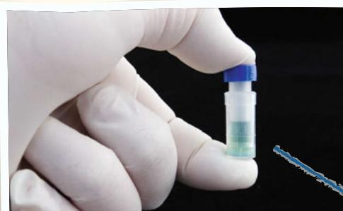
4. Press down plunger completely to filter sample
