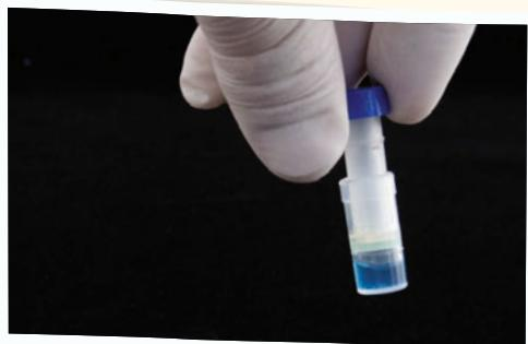
3. Next, insert Plunger, press half way down and shake or swirl to extract compound from silica gel.
