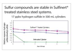
reacting with or adsorbing to the steel. These Swagelok® high pressure sample cylinders are Sulfinert® treated for greater stability of sulfur compounds and mercury. DOT rating to 1,800 and 5,000 psig allows sampling at gas wellheads as well as in the refinery. Use of high pressure sample cylinders is cited in ASTM D1265, Standard Practice for Sampling Liquefied Petroleum (LP) Gases, Manual Method.
