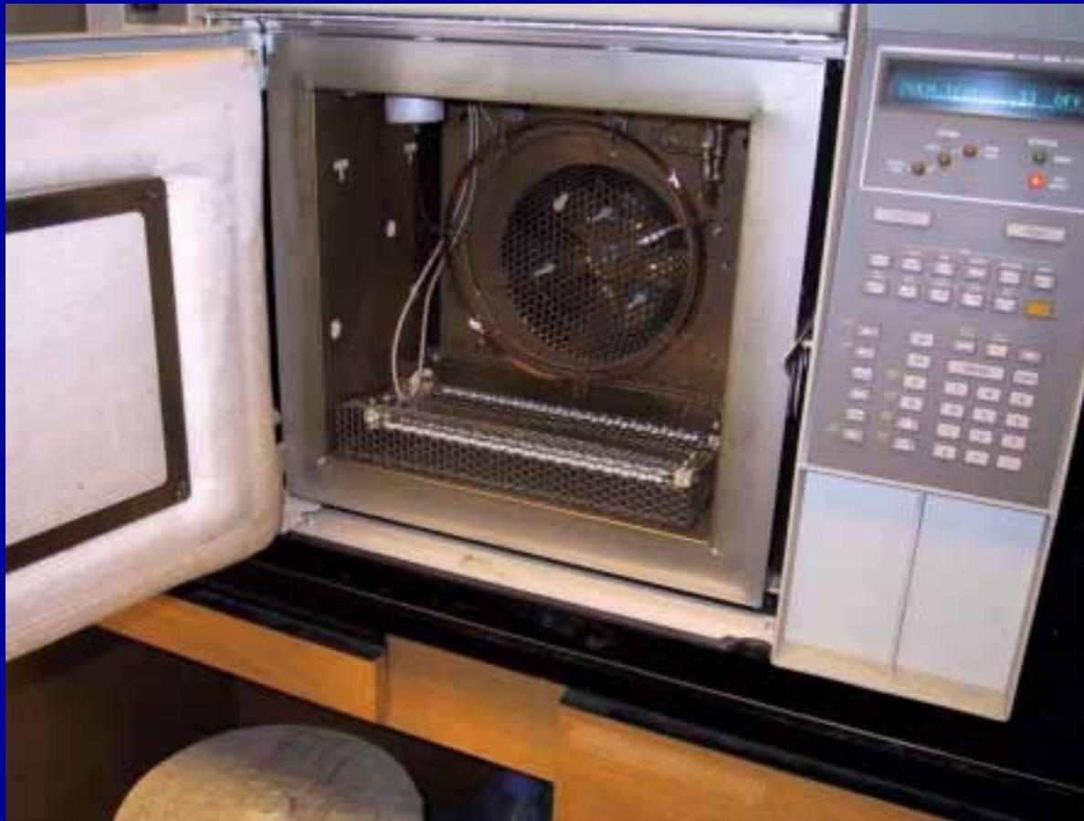
**GC Racer Heater Installed in an Agilent 5890**
