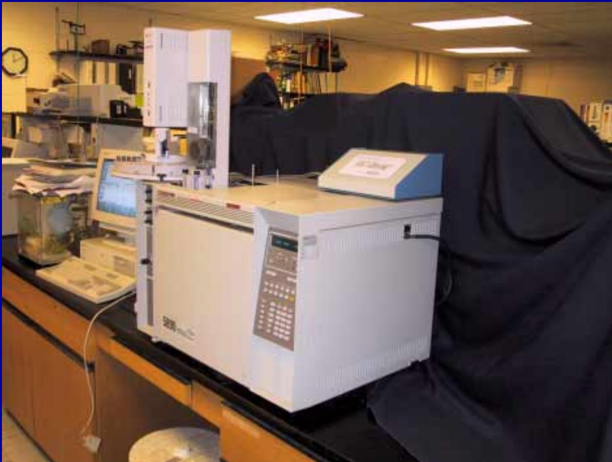
GC Racer Installed on an Agilent 5890
