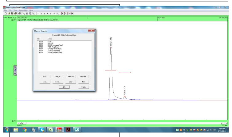
In this chromatogram Relay G was turned off at 4 minutes which allowed the TCE to appear but not ( or mostly not ) the PCE peak. By adjusting the Relay G off time by trial and error you can control which peaks make it onto the analytical column.
