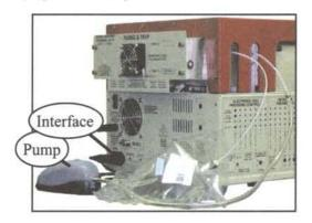
Typically, the vacuum pump is used to draw gaseous samples through the traps for ambient air monitoring applications, or to load the loop of a gas sampling valve by pulling sample gas from a remote location.
