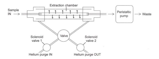
When the sample is pumped through the gas extraction loop, the dissolved gases permeate through the membrane into the extraction chamber. Solenoid valves are included for purging the gas extraction loop with helium between runs.
