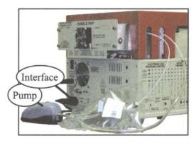
Typically, the vacuum pump is used to draw gaseous samples through the traps for ambient air monitoring applications, or to load the loop of a gas sampling valve by pulling sample gas from a remote location.
