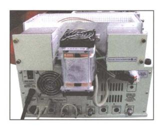
The CryoCooled Peltier Trap is basically a heated trap sandwiched between two Peltier coolers. The CryoCooled Peltier Trap also requires a 10-port gas sampling valve (not included). While the Peltier Trap is enriching the
