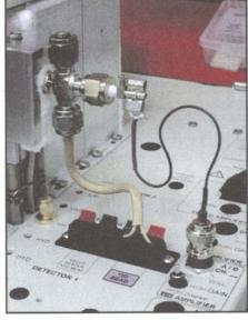
The TID is similar in design to the FID and NPD. The electrically heated thermionic bead (TID bead) is positioned so that the column effluent contacts the hot bead surface. Analyte molecules containing NO2 (nitro) functional groups such as TNT (trinitrotoluene) undergo a catalytic surface chemistry reaction. The resulting ions are attracted to a collector electrode, amplified, and output to the data system.
