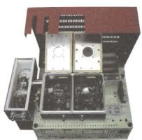
The Virtual Oven™ is optionally available on the 8610C, 8610D and 310 GC 3) chassis; use part number 8690-1000 to request it in place of an airbath column oven. The Virtual Oven™ provides for the programmable heating and very rapid cooling of a 1/8" OD packed column up to two meters in length. Using low voltage AC to resistively heat the column, the column itself becomes the heater. The advantages of the Virtual Oven<sup>TM</sup> are:
