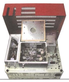
This BTU GC is customized with an FID detector, an additional gas sampling valve, and a built-in 4 channel PeakSimple data system.
