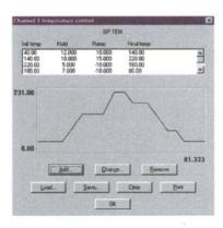
Program one or two SRI GC column ovens from ambient to 400°C with unlimited ramps and holds, 0.01 degree resolution, and negative programming.
