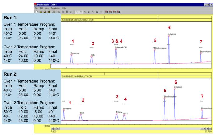
As seen in the Oven 2 temperature program for Run 2, PeakSimple provides negative programming capability in addition to unlimited ramping. Making this slight change in Oven 2's temperature program not only separated Tolene and PCE, it also altered the retention times of Ethylbenzene and o-Xylene. The TCS GC gives you the power to move peaks!
