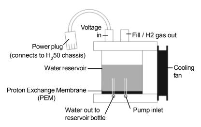
Operational Diagram of the H<sub>2</sub>50 Generator Cell
