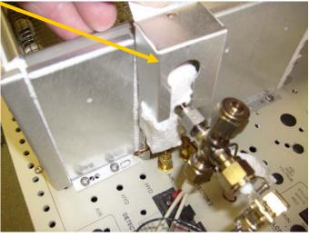
The methanizer jet may be repacked many times. Use a stiff wire to poke the old catalyst/glass wool out of the jet.
