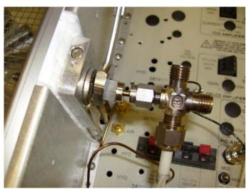
Re-connect the ignitor, collector electrode and cap to the detector body.
