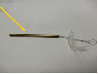
Use some thicker, stiffer wire ( or a piece of metal wide bore capillary column ) to position the glass wool plug halfway down the jet.
