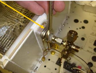
The FID/Methanizer body is different from the regular FID body because the jet is remove-able on the FID/Methanizer version.
