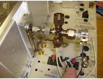
Set the methanizer ( detector block ) temperature between 300 and 380C depending on the sensitivity required.
