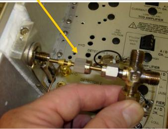
Tighten the jet in the bulkhead fitting using a 7/16" wrench.
