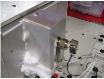
The cannabinoid molecules, \( \Delta 9-THC, CBD, \) and CBN (and for more advanced operators, CBC, \( \Delta 8-THC, \) and CBG) are separated by a 15-meter metal capillary column which is heated in the column oven.
