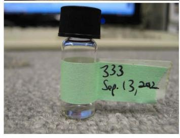
Rinse the syringe first then use the 10ul syringe delivered with the GC (SRI #8670-9550) to withdraw 2-3ul of the working standard. Puncture the septum rather than open the vial to avoid letting the methanol solvent evaporate each time the vial is opened. Pump the plunger several times to get rid of air bubbles.
