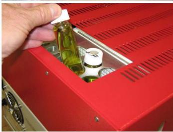
The GC includes SRI's Flame Ionization Detector (FID) which is able to measure the cannabinoid molecules based on its ability to detect the combustion of hydrocarbon molecules.
