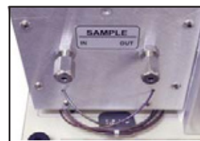
Room Temperature Silcosteel sample loop
