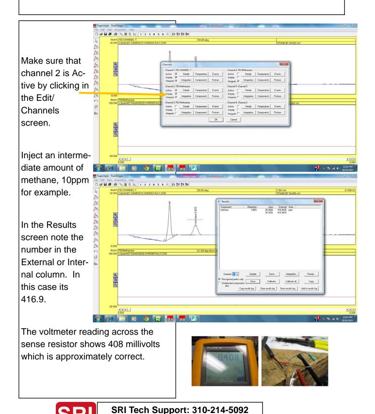
Note that the 4-20ma output only changes at the end of an analysis, and that the current is held constant during the subsequent analysis and only updated once the next analysis is complete.
