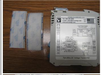
Tape the Velcro to the side of the Acromag which does not have the circuit diagrams.
