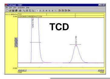
This chromatogram is from a direct injection of 0.5mL of human breath. The longer we hold our breath, the higher the CO<sub>2</sub> content. This was the result of a class experiment called "Waiting to Exhale," which is included in the manual. It is a contest to see who can blow the most CO<sub>2</sub>. Participants merely exhale into a 3mL syringe, then inject 0.5mL into the on-column injector of an Educational TCD GC.
