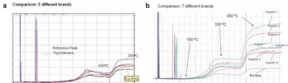
Figure 2 Bleed comparison of different types of 5% diphenyl and aryl phases: a) 0.25- $\mu$ m film, b) 0.5- $\mu$ m film.
