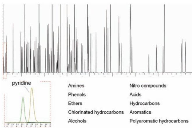
Figure 10 A multicomponent environmental analysis such as U.S. EPA 8270 is usually analyzed using an Rxi-5Sil MS column. All groups of compounds elute as symmetrical peaks. (See Table 3 for conditions.)
