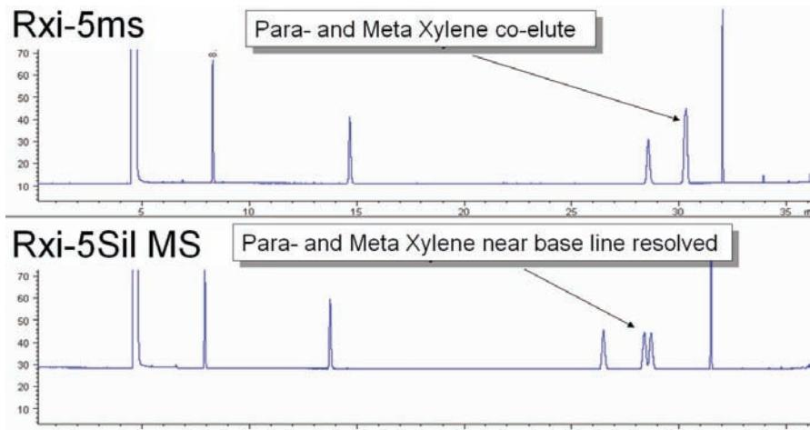
Figure 8 Separation of xylenes on Rxi-5ms and Rxi-5Sil MS columns, both  $60\text{ m} \times 0.25\text{ mm}$ ,  $df = 0.25\text{ }\mu\text{m}$ , temperature =  $35^\circ\text{C}$ .
