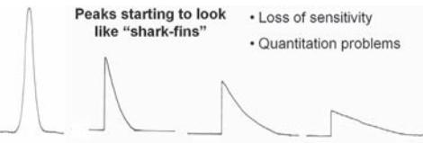
Figure 3 The typical peak shapes seen when adsorption in the column occurs.
