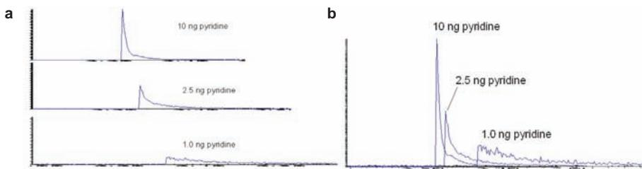
Figure 6 Impact of the amount of active compound injected on retention time and peak shape. Peak shown: pyridine at 10, 2.5, and 1 ng on a conventional state-of-the-art column (30 m × 0.25 mm, df = 0.25 μm). a) Individual runs, b) overlaid chromatograms.
