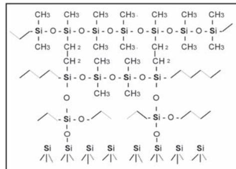
Figure 1 Schematic representation of Rxi bonding process (cross-bonding, surface bonding, deactivation, and shielding for minimization of impact of [re]active silanols).
