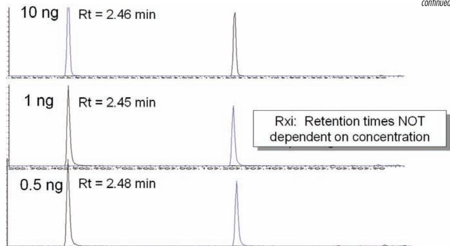
Figure 7 Peak shape and retention of 10, 1, and 0.5 ng pyridine on similar column dimensions as in Figure 6, using Rxi column technology.
