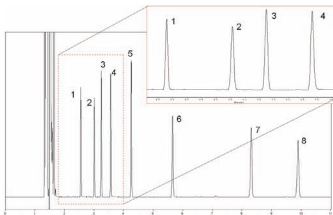
Figure 9 Standard test of Rxi-5Sil MS columns. Column:  $30\text{ m} \times 0.25\text{ mm}$ ,  $df = 0.25\text{ }\mu\text{m}$ . 1) 2,6-hexanediol, 2) 4-chlorophenol, 3) methylnonanoate, 4) 1-decyldamine, 5) tridecane, 6) undecanol, 7) acenaphthylene, 8) pentadecane.
