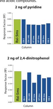
Figure 2 Analyte levels in samples are unknown; only inert columns, which prevent concentration from affecting retention time, can assure accurate results.
