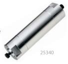
The ASI FlatLine Pulse Damper combines performance and reliability in a simple, easy-to-use housing. Standard 10-32 inlet and outlet ports allow quick connection into virtually any HPLC system. Solid core technology provides reliable long-term operation without the downtime associated with ruptured or leaking membrane dampers.  $600-700~\mu L$  internal volume at ambient pressure. Maximum pressure: 6,000~psi~(41,369~kpa)
