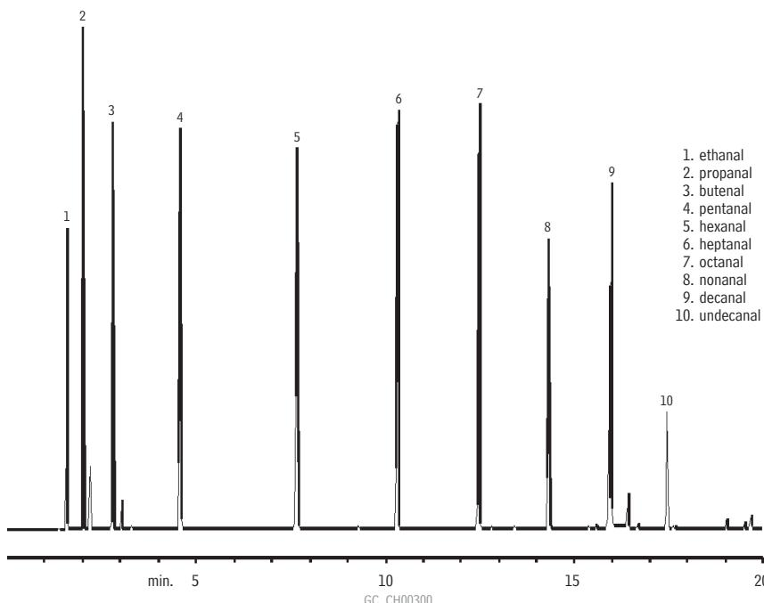
Column: Rtx®-Wax, 30m, 0.25mm ID, 0.50 $\mu\text{m}$  (cat.# 12438)
