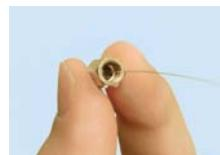
The ferrule will be properly seated and should remain in place when light force is applied. Install the column into the GC/MS interface.
