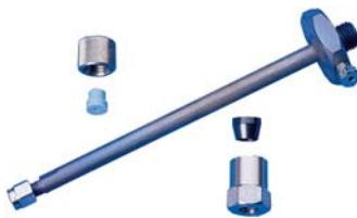
Our low-volume injector can be installed in a matter of minutes. Remove the septum nut or splitless weldment and insert the Restek low-volume injector through the split injector. Tighten the base nut and you're ready! Includes a 1/16-inch nut, a 1/16-inch ferrule, a base nut and 1/4-inch Vespel®/graphite ferrule, a 1/16-inch capillary nut, a 5-pack of low-bleed plug septa, and a low-mass septum nut. Order appropriate capillary ferrules separately.
