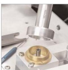
Easily loosen the nut by aligning the two pins on the bottom of the wrench with the two open slots on the nut...
