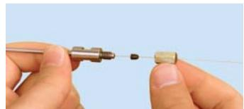
Install the nut and ferrule onto the column, then insert the column through the installation tool, exposing several centimeters at the exit end. Tighten the nut.
