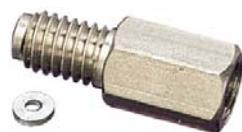
Agilent's MSD interface uses a butt-seal to simultaneously seal the MSD source to the capillary column. This system is prone to leakage. Restek's MSD conversion fitting is designed with two separate seals to reduce the chance of leaks: a crunch washer seals the MSD conversion fitting to the source; a ferrule seals the capillary tubing to the conversion fitting.
