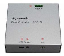
① Motor connection terminal (CH1): B/B /A/A
