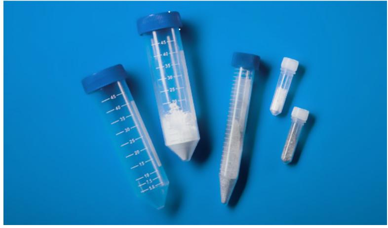
QuEChERS Tubes For Extraction and Clean-Up of Pesticide Residues From Food Products Convenient, ready to use centrifuge tubes with ultra pure, preweighed adsorbent mixes.
