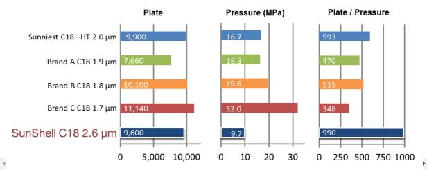
Column: 50 x 2.1 mm C18, Mobile phase: Acetonitrile/water=(70/30), Temperature: 25 °C
