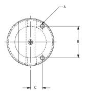
Mounting holes can be provided in the shell on top of the valve. Please consult Bio-Chem Valve and Omnifit concerning top mounting holes.
