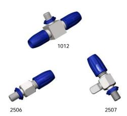
Omnifit variable bore adaptors allow any size of tubing between 0.5 and 4mm O.D. to be connected to a 1/4"-28 UNF port via the 'Omnifit Cap'. The valved version has a Tefzel® rotor. Each adaptor has a male 1/4"-28 UNF thread that will fit any female 1/4"-28 UNF threaded port.
