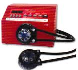
Peristaltic pumps have few moving parts. Their lack of valves, seals and glands make them inexpensive to maintain - especially with our interchangeable heads and tubes. Fluids can be kept more clean and sterile than other pumping methods.
