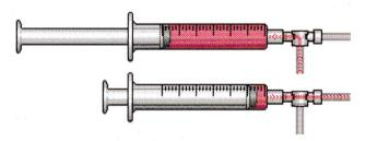
Alternate dispenses of two chemicals. Automatically alternates between two pumps. Pump chemical 1 – then chemical 2, then repeat.
