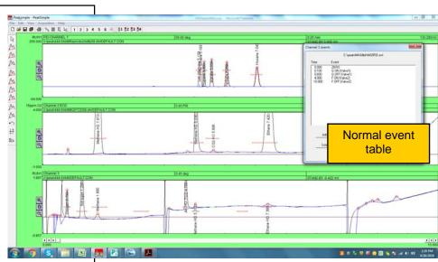
This chromatogram shows the same sample but with Valve 1 and 2 injected simultaneously. Relay A is turned ON at the same time (.1minute) which stops the carrier gas flow in the Haysep and capillary columns. This creates some extra "ghost" peaks but does not substantially affect the anal-
