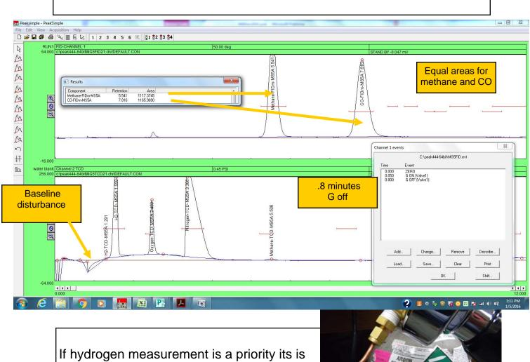
If hydrogen measurement is a priority its is best to use Argon carrier gas instead of helium. Because there is an un-avoidable baseline disturbance when Relay G turns off and backflushes the pre-column, it may make sense to use a 6 foot MS5A column instead of the 3 foot MS5A column. The 6' column makes the Hydrogen peak come out a little later giving the baseline a chance to stabilize before the H2 peak begins.
