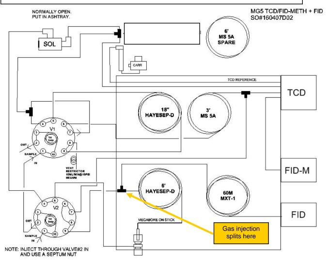
1) This drawing shows a capillary column set up for gas injection from the gas sampling valves onto both the Haysep and capillary column.
