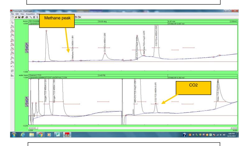
This is room air which has 2ppm of methane, 400ppm of CO2 and 10,000ppm of water.
