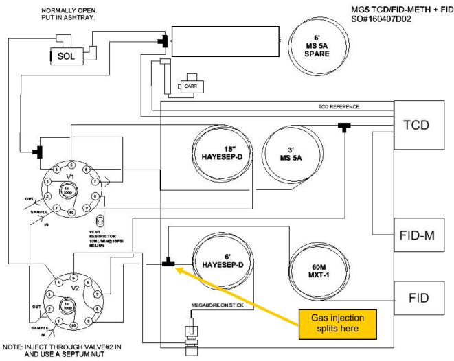
1) This drawing shows a capillary column set up for gas injection from the gas sampling valves onto both the Haysep and capillary column.
