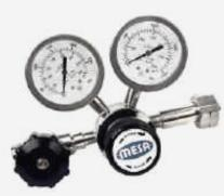
Brass bodies are recommended for non-corrosive gases. Chrome plated brass bodies are also recommended for non-corrosive gases. The addition of chrome plating to the brass body helps to protect the outside body of the regulator from corrosive ambient conditions such as found in chemical plants and refineries. 316L Stainless Steel bodies are
