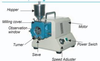
The fixed knife and revolving knife cut the materials into small pieces without reducing its water content. applicable for grain, seeds, plastic fibers, and leathers, size of the particles is controlled by the sieve under the mill pot.
