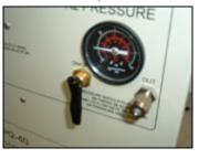
tion of soap and water. If tiny bubbles appear around the base of a fitting, then tighten that fitting just a little. You may have to remove the bead of silicone sealant to get your wrench on the fitting. The plastic parts can crack if too much pressure is applied so tighten just enough to stop the leak.
