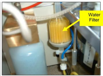
This filter is readily available in most countries of the world. Be sure to use a filter which is all plastic ( no metal ) to avoid poisoning the membrane.
