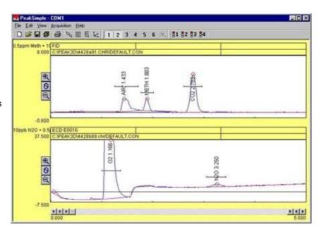
The Greenhouse GC is not limited to  $CO_2$ ,  $CH_4$  and  $N_2O$ . The FID-Methanizer detects hydrocarbons as well as CO and  $CO_2$  (as methane). The sensitive ECD detector responds to electronegative compounds, especially chlorinated, fluorinated, or brominated molecules like PCBs and pesticides. With a low-volume sample loop, the Greenhouse GC can be used to measure gases produced by bacterial metabolic processes and life cycles.
